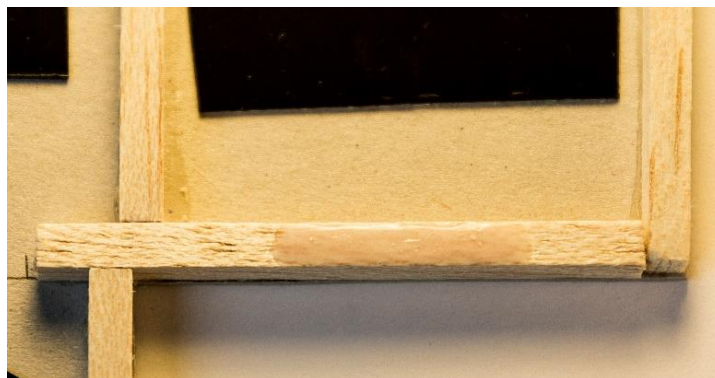
Figure 12: Nail polish trace for windows on the basal wood strips.
